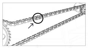
The engine is operating, the gearbox shifts, but there is no motion on any of the transmissions — there may be a break in the central chain.
