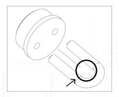
In order to unscrew the cap of a wheel tank, insert an extender into the wrench (screwdriver etc.).
