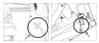
The clutch limit switch may be faulty.
