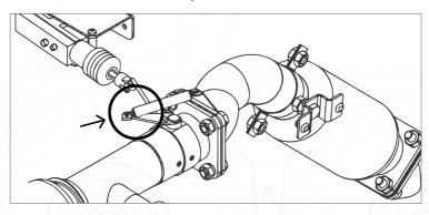
Inflation valve on the exhaust pipe is closed.
