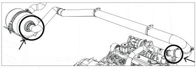
Water has gotten into the air hose and filter.
